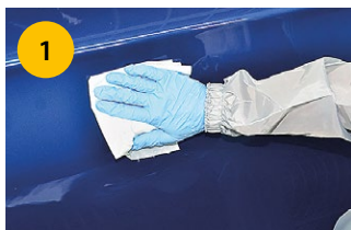
1 Degrease and wipe clean. Use Mirka Tack cloth.
